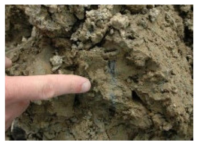
Figure 5. Blue/grey or orange mottling in the soil is an indication of poor drainage.
