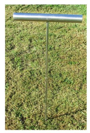
Figure 16. Soil probe.
