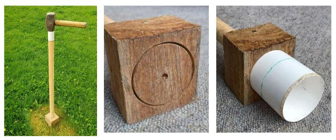
Figure 14. 'Fancy' ring driver, with 4 cm deep slot cut in a wood block with hole saw, that the ring snugly fits in with a thick wood shaft to allow ring to be driven from standing position.
