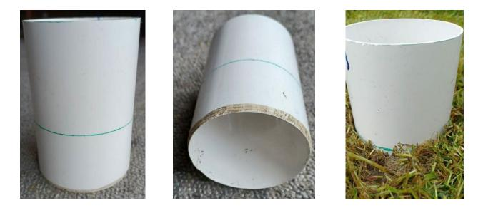
Figure 11. Ring infiltrometer made from 12 cm long, 8 cm diameter guttering down pipe, showing sharpened end for driving into soil and inserted into the soil to the depth mark.
