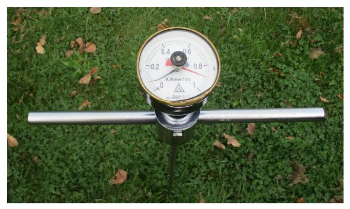
Figure 17. Soil penetrometer.
