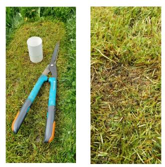
Figure 12. Ground preparation – clearing as much vegetation and residue from the test location as possible.
