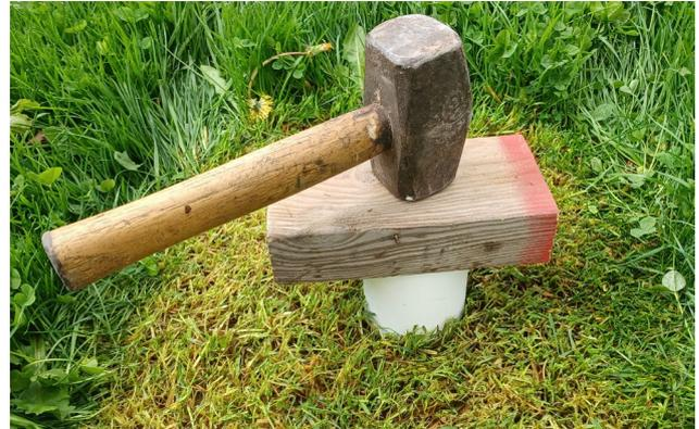
*Figure 13. Simple method for driving ring into ground – wooden batten and club hammer.*
