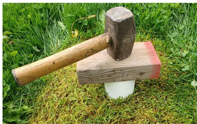
*Figure 13. Simple method for driving ring into ground – wooden batten and club hammer.*
