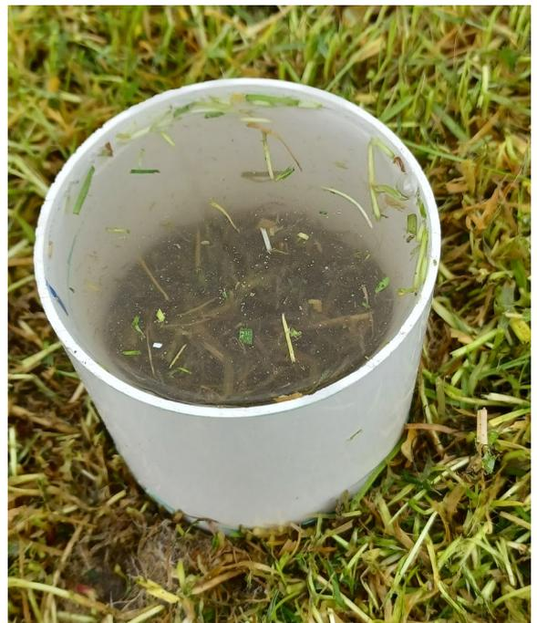
Figure 15. Infiltration ring filled with water.
