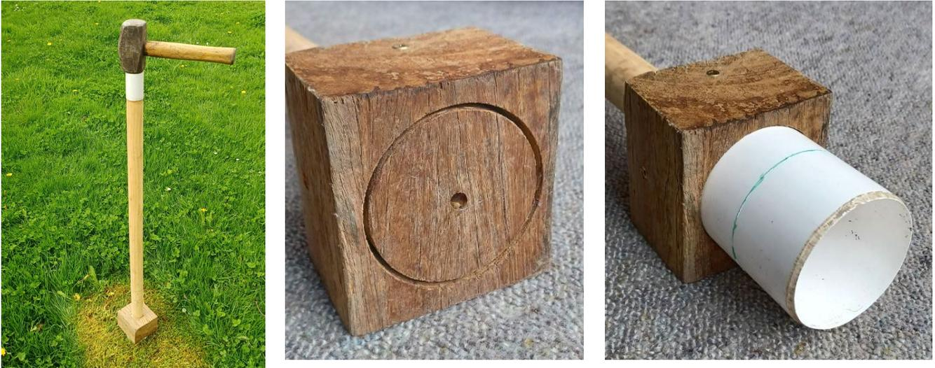
Figure 14. 'Fancy' ring driver, with 4 cm deep slot cut in a wood block with hole saw, that the ring snugly fits in with a thick wood shaft to allow ring to be driven from standing position.
