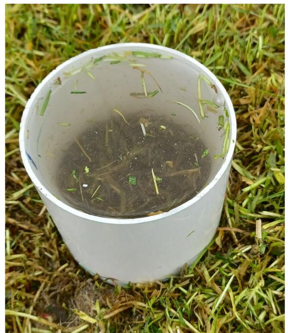
Figure 15. Infiltration ring filled with water.
