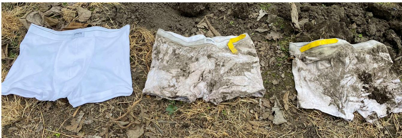
*Figure 8. Decomposition comparison. Fresh cotton undies (left), a pair buried for 24 days (centre) shows mild decomposition, while a pair buried for 51 days (right) shows holes due to decomposition.*
