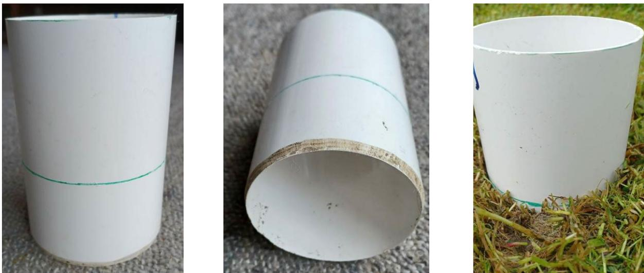
*Figure 11. Ring infiltrator made from 12 cm long, 8 cm diameter guttering down pipe, showing sharpened end for driving into soil and inserted into the soil to the depth mark.*
