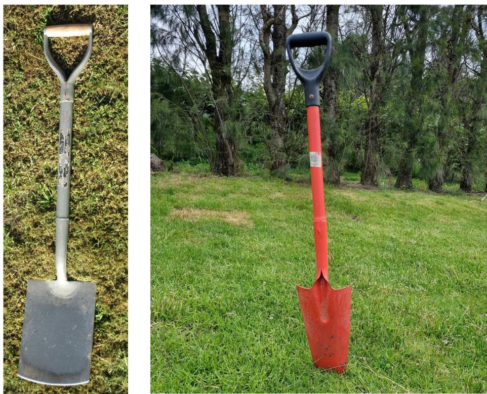
*Figure 4. Standard spade left and post hole / ditching spade right.*
