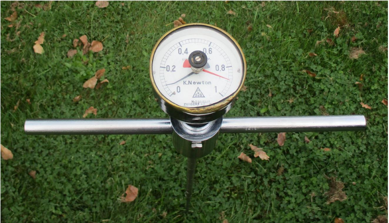
Figure 17. Soil penetrometer.
