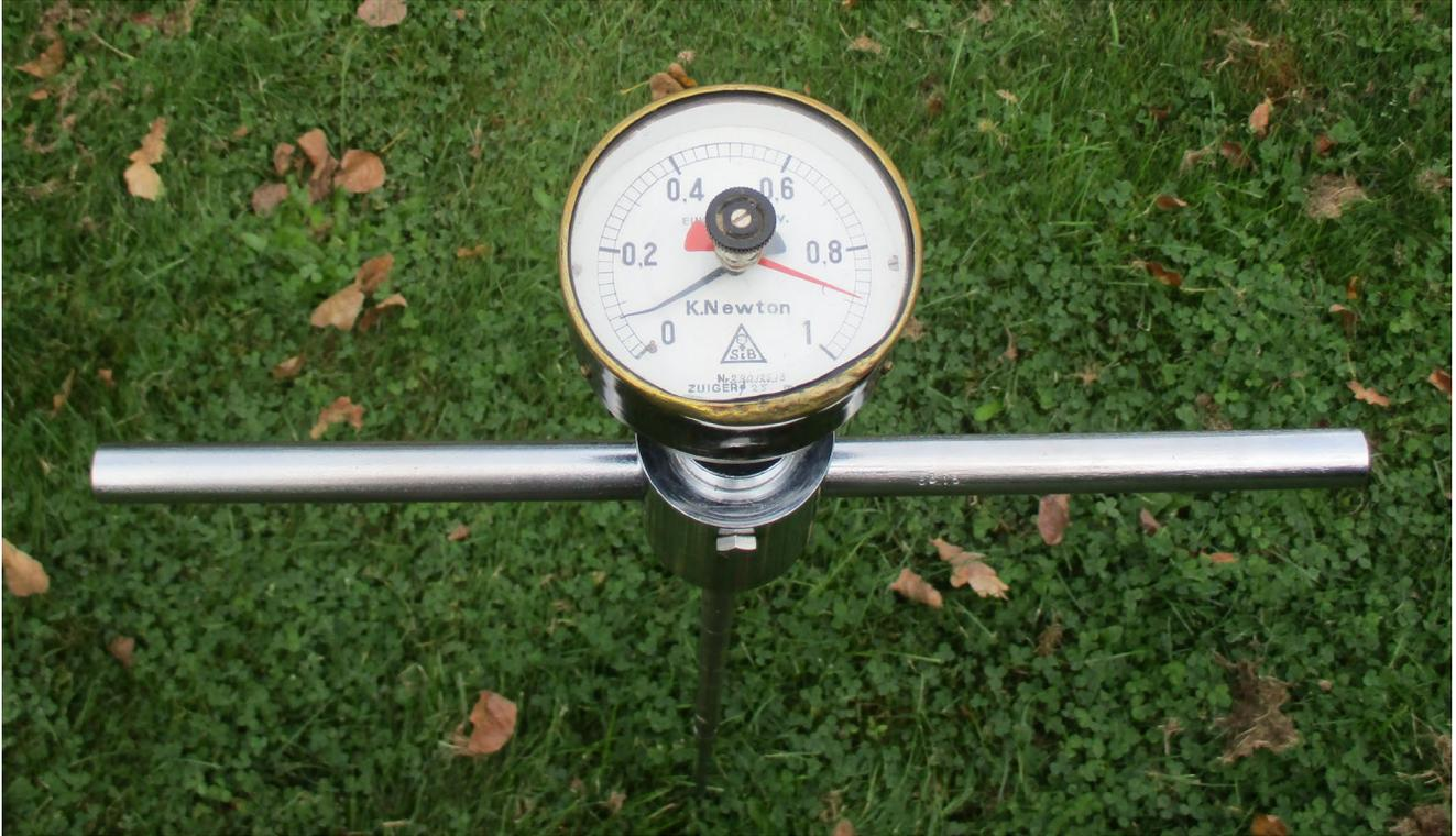
*Figure 17. Soil penetrometer.*
