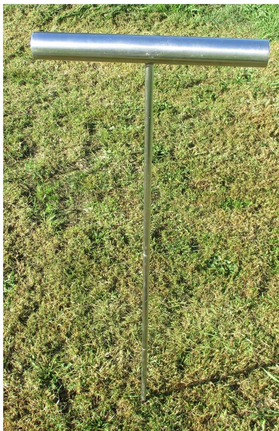
Figure 16. Soil probe.
